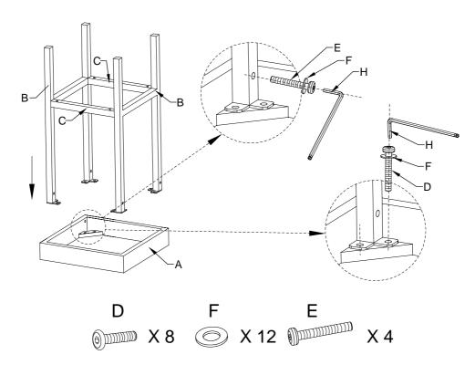
Step 3. Using bolts (D), and washers (F) attach stretchers (C) to foot panels (B).
